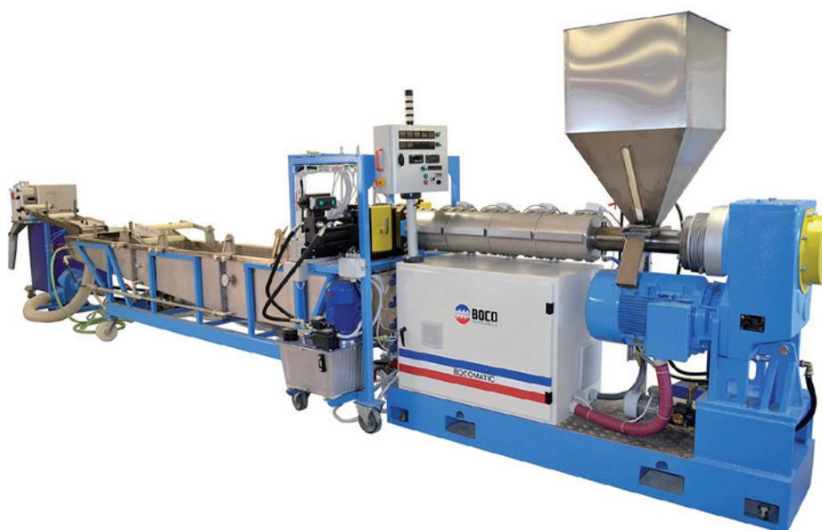
We offer complete strand pelletizing lines that will fully meet your requirements. Thanks to their flexibility can process a wide range of rigid plastic crushed material PP, PA, PE, PC and others. Our lines are known for their reliability, modern technology, excellent quality of the cutting tools, flexibility, consistent outstanding of pellets quality and economical production. Operation of the machines is in the maximum possible extent user-friendly and controlling is intuitive.
